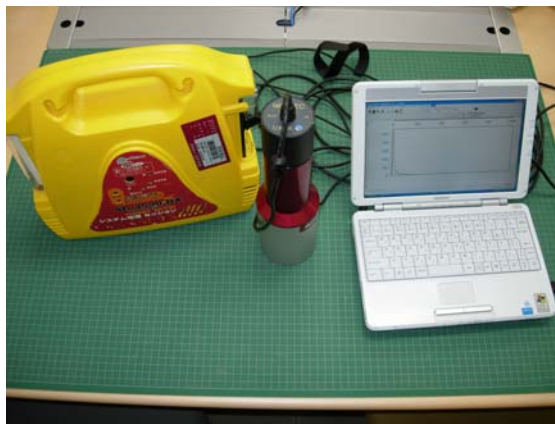
Figure 3: Instrumentation for natural gamma-ray survey
